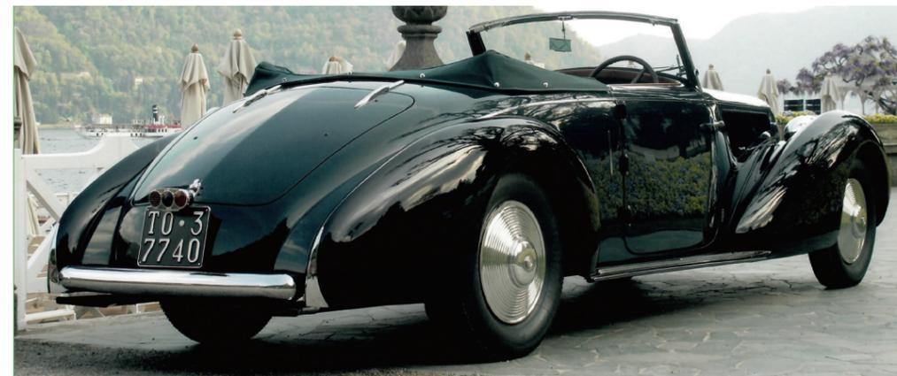
*New car had a 3.0-litre engine, the option of an electric soft-top and hydraulic brakes.*
