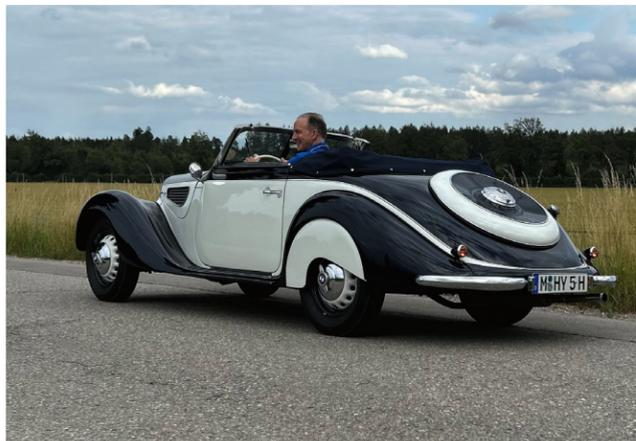
BUILT BETWEEN 1937 AND 1941, THE BMW 327 WAS A rare car – just 1304 examples were ever made. It was powered by a water-cooled six-cylinder engine with two Solex downdraught carburetors. Its 2.0-litre capacity provided 55bhp, enough to propel the BMW to 125km/h. The motor benefitted from a light-alloy cylinder head with overhead valves and a side camshaft operated with pushrods and rocker arms. When new, the 327 cost a hefty 7500 Reichsmarks.
