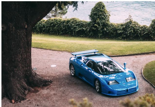
THE BUGATTI EB110 WAS AN ABSOLUTE PIONEER IN the supercar class. Not only did it have a carbonfibre tubular frame built in collaboration with the French company Aérospatiale, but it was the first 'hypercar' to employ permanent four-wheel drive, successfully deploying the 610bhp unleashed from its 3.5-litre quad-turbo V12 engine. Its lap record of seven minutes and 44 seconds on the Nordschleife in 1993 was only equalled in 2002.
